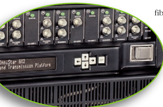
The optional shelf door with display unit and navigation buttons (shown here) provides both a fiber management solution and a local status monitoring and control interface.
