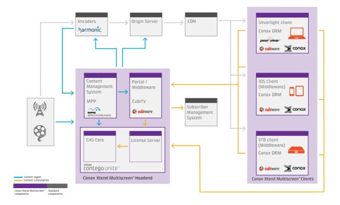
Figure 1 Conax Xtend Multiscreen<sup>™</sup> high-level architecture
